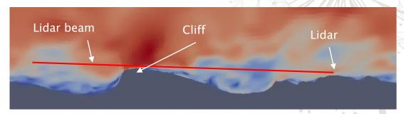
Schematic display of validation case, measuring flow recirculation and turbulence downwind a steep cliff using a high-resolution lidar system capable of measuring small scale turbulence at up to 2000 meter distance
