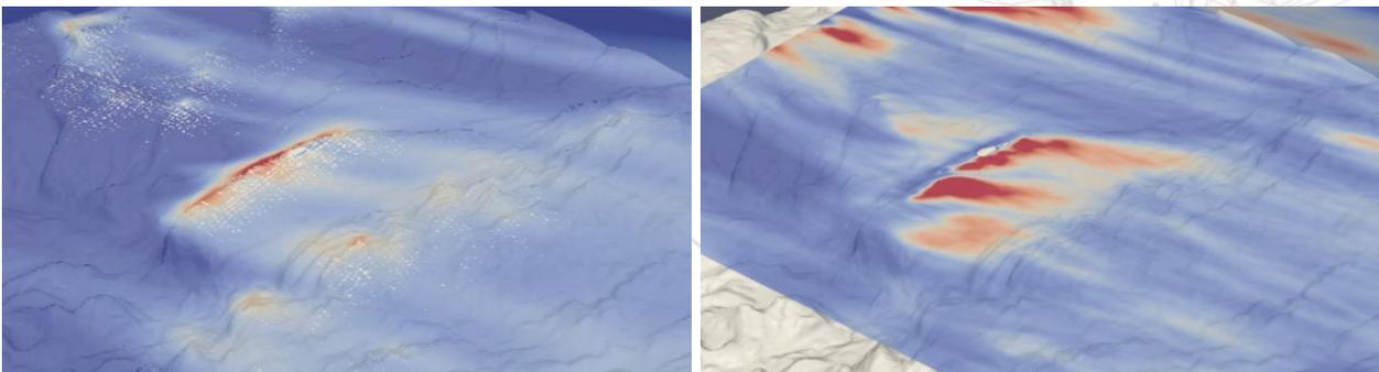
RANS model (left) shows clear underprediction of turbulence behind cliff. DES model better describes the physics of large scale recirculation
