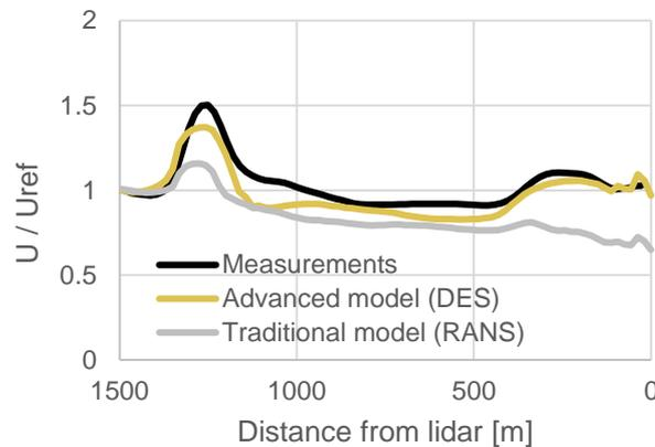
Model validation along a lidar line-of-sight clearly show shortfall of traditional RANS model in highly complex terrain. RANS model gives error in the order of 40%!
