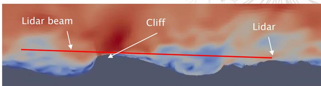
Schematic display of validation case, measuring flow recirculation and turbulence downwind a steep cliff using a high-resolution lidar system capable of measuring small scale turbulence at up to 2000 meter distance
